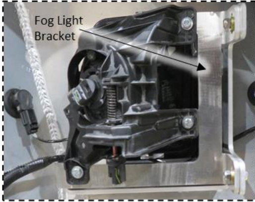
Figure 5a: OEM fog light installation
