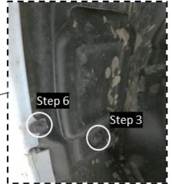
Figure 1c: Accessing the Headlight Tab & Fender fastener Removal (Driver Side shown)
