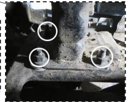
Figure 1e: Bumper Fastener Removal (Driver Side shown)
