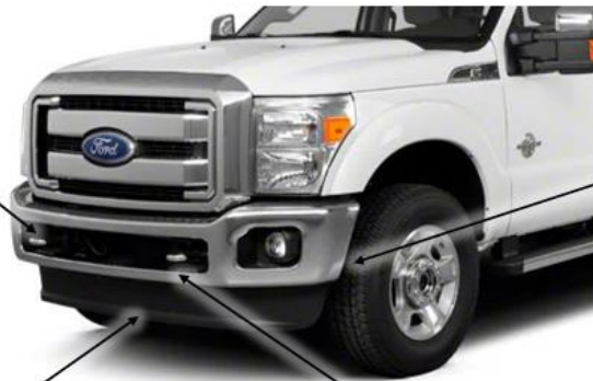
Figure 1d: Remove OEM tow loops and lower frame extensions
