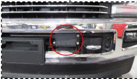
Figure 1b: Remove CAS Radar (if applicable)
