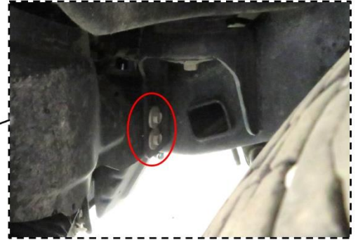
Figure 1a: Remove rear fasteners (Driver Side shown)
