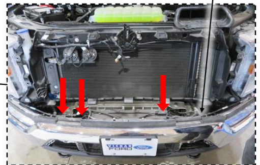
Figure 1d: Remove front grille
