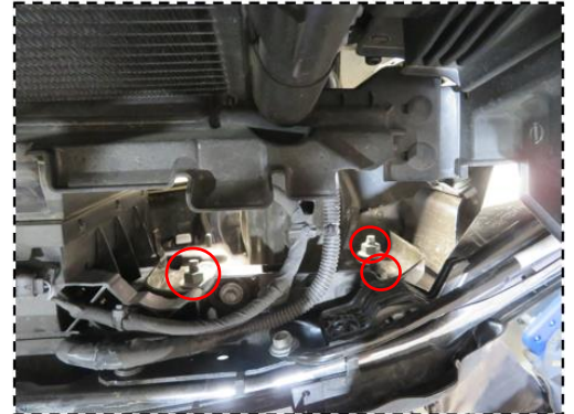
Figure 1e: Remove bumper bolts (driver side shown)
