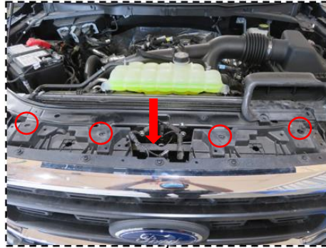
Figure 1c: Remove radiator cover
