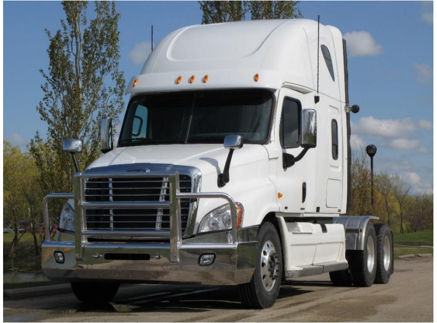
Figure 12 – Herd Truck Guard Installed
