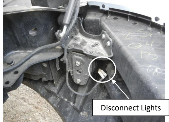
Figure 3 – Factory Driving Lights Disconnected (Passenger Side Shown)
