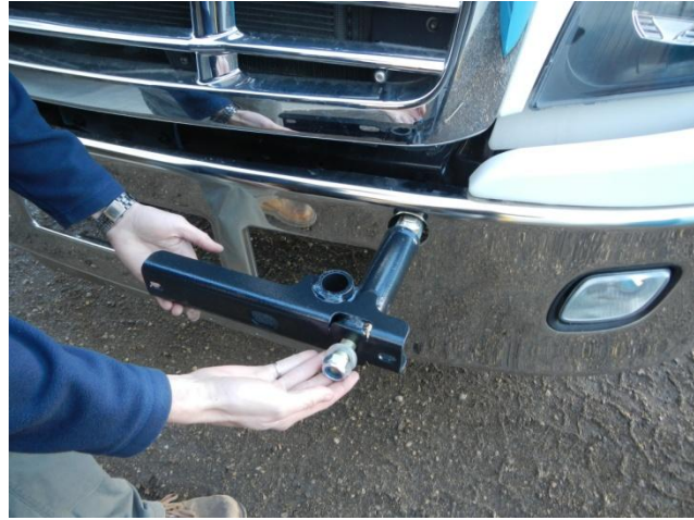
Figure 3 – Submount assembly installation.
