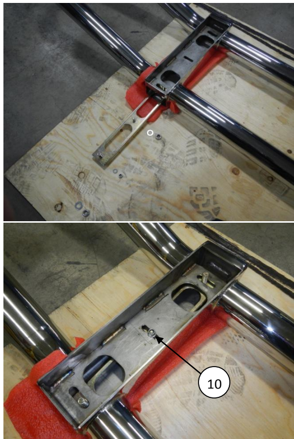
Figure 2 – Guard mounting plate installation.
