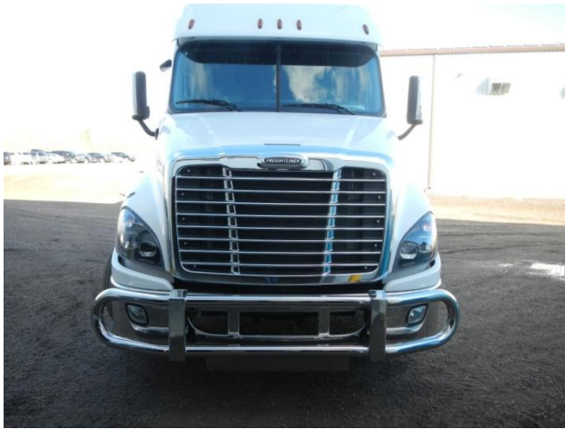
Figure 6 – Bumper guard installed (Narrow Rad version shown).
