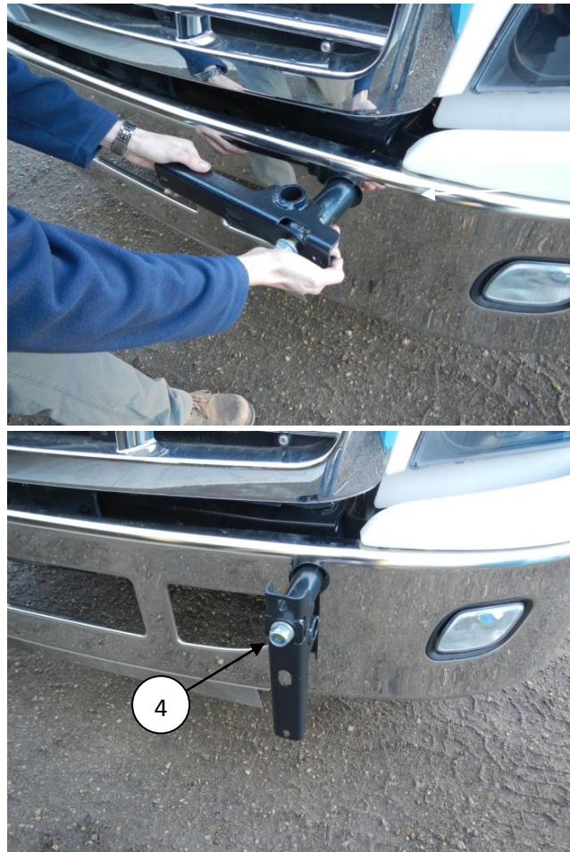
Figure 4 – Submount assembly installation. Narrow Rad version shown.
