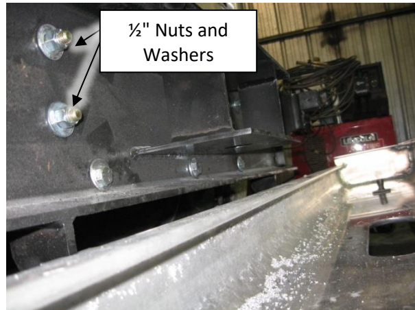
Figure 8 – HERD Bracket Installation
