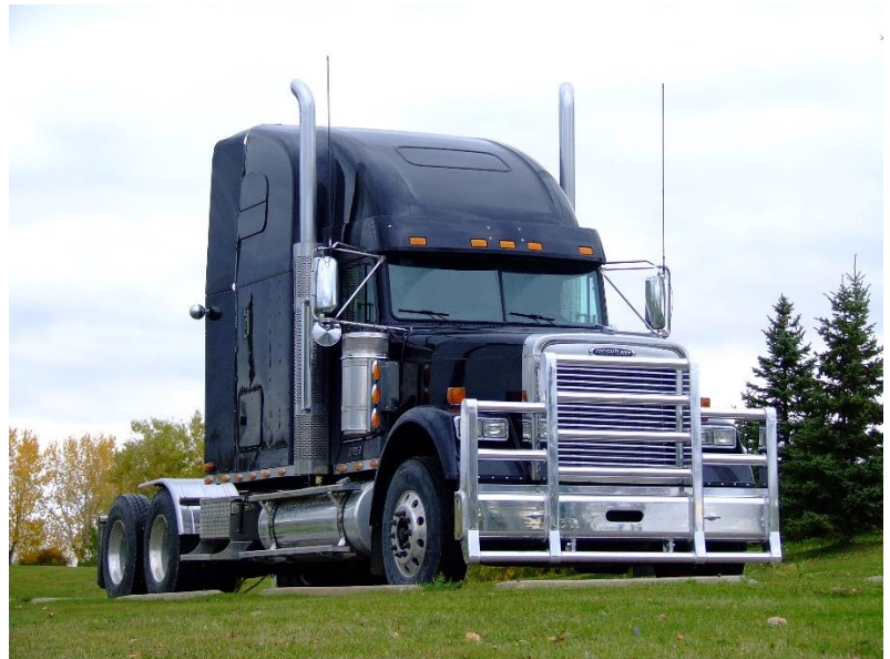
Figure 10 – Herd Truck Guard Installed
