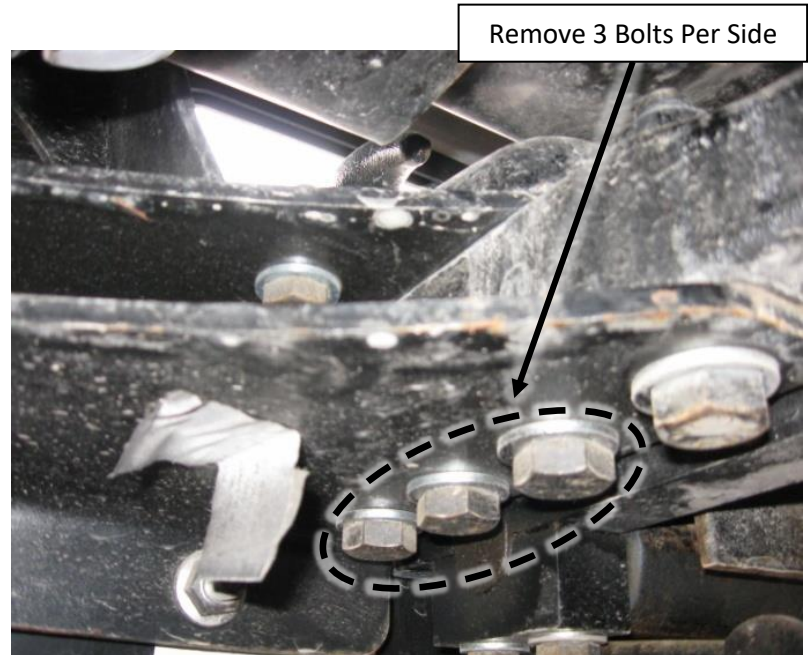
Figure 4 – Tow Hook Removal (Driver Side Shown)
