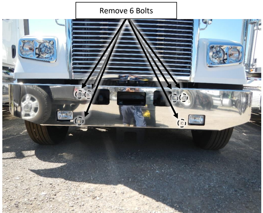
Figure 3 – OEM Bumper Removal Front View
