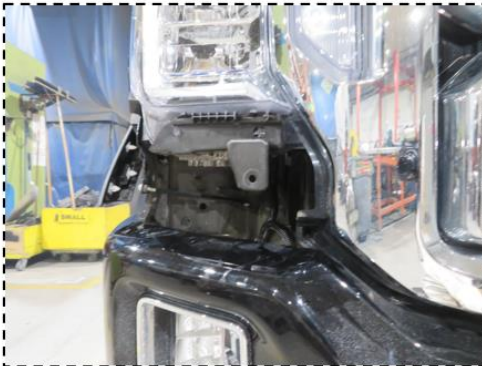
Figure 1e: Remove valance (passenger side shown)
