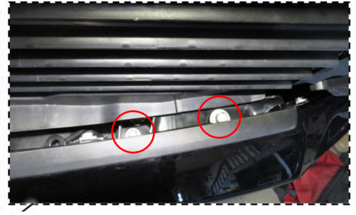
Figure 2d: Remove bumper fasteners (driver side shown)
