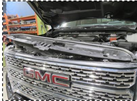
Figure 1b: Remove radiator cover
