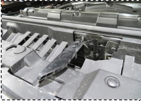
Figure 1a: Remove latch handle
