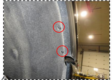
Figure 1c: Remove fender liner screws (passenger side shown)
