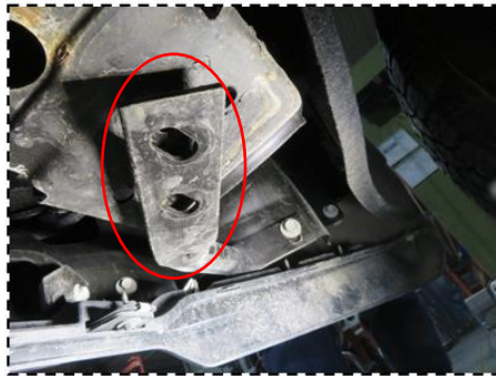
Figure 2c: Bottom fasteners location (passenger side shown)
