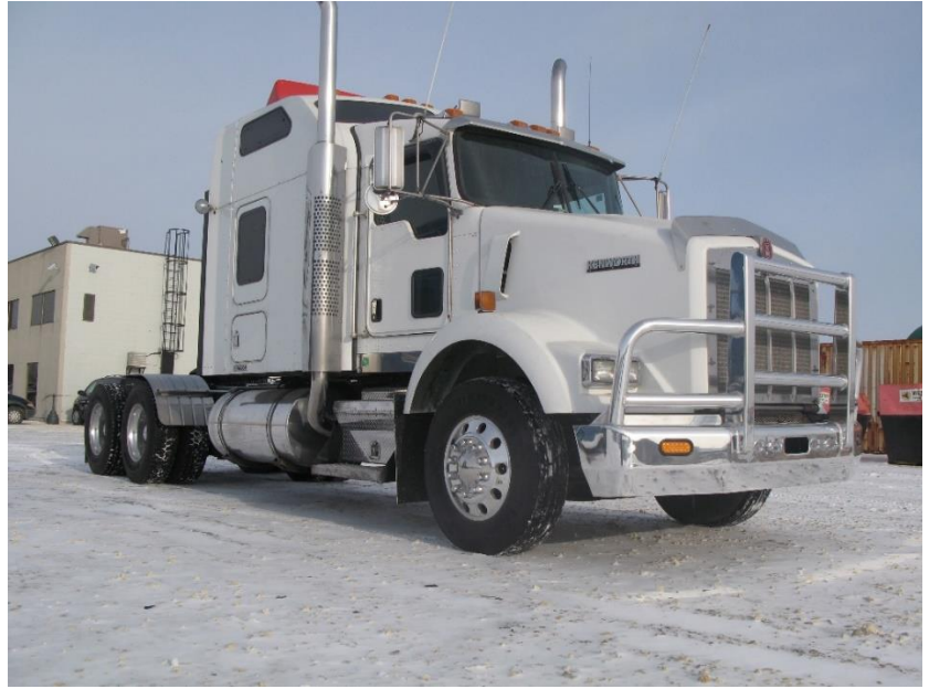
Figure 12 – Herd Truck Guard Installed
