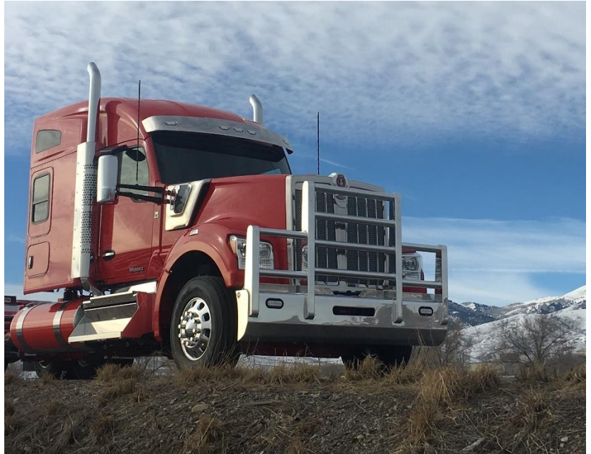
Figure 9 – Herd Truck Guard Installed
