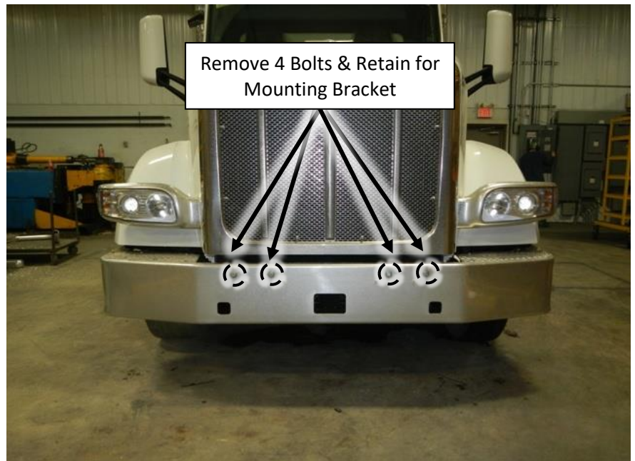
Figure 3 – OEM Bumper Removal Front View.
