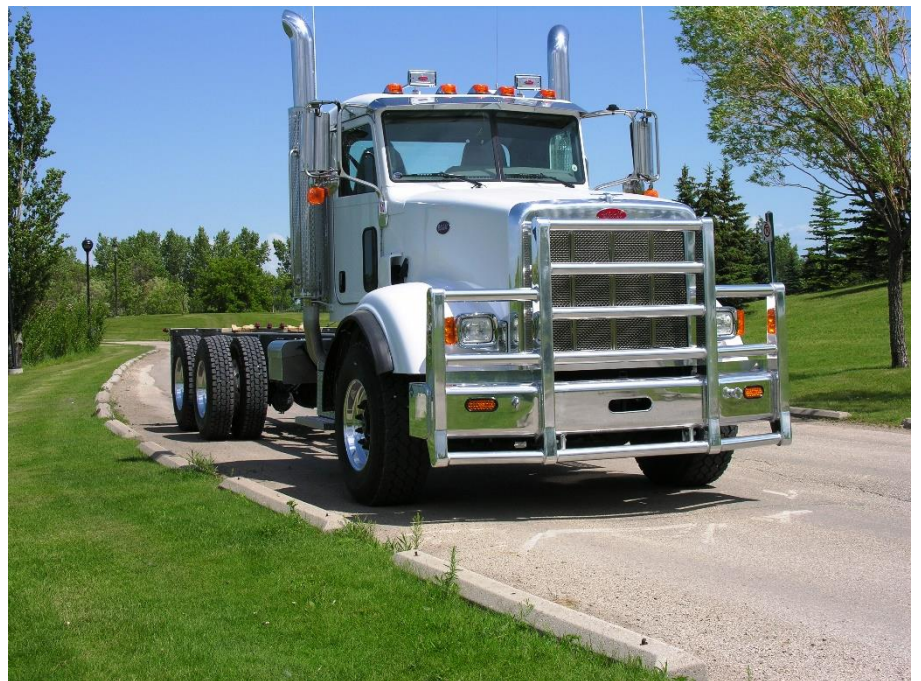
Figure 10 – Herd Truck Guard Installed
