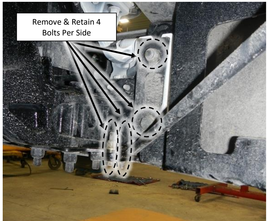
Figure 4 – OEM Bumper Removal Back View (Passenger Side Shown)
