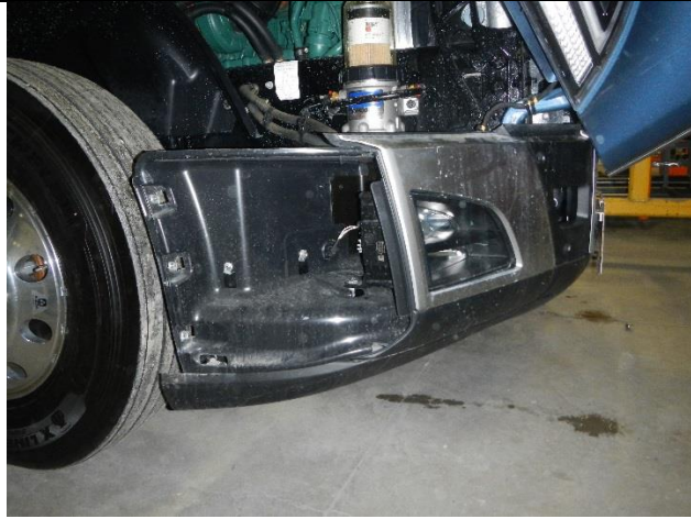
Figure 1 – OEM Driving Light Uninstall (Passenger Side Shown)
