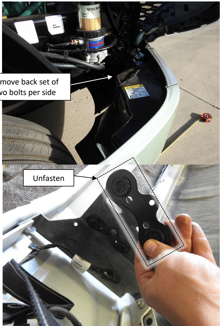
Figure 2 – OEM Bumper Uninstall (Passenger Side Shown)
