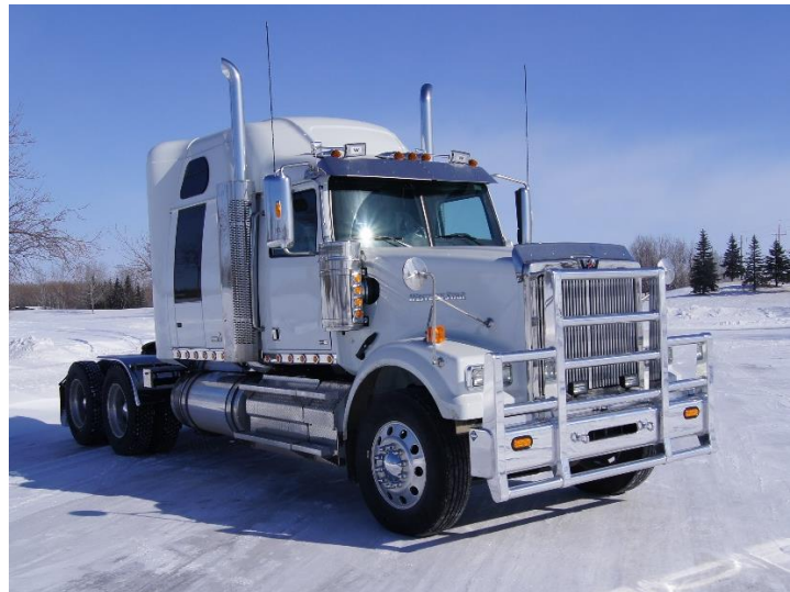
Figure 10 – Herd Truck Guard Installed
