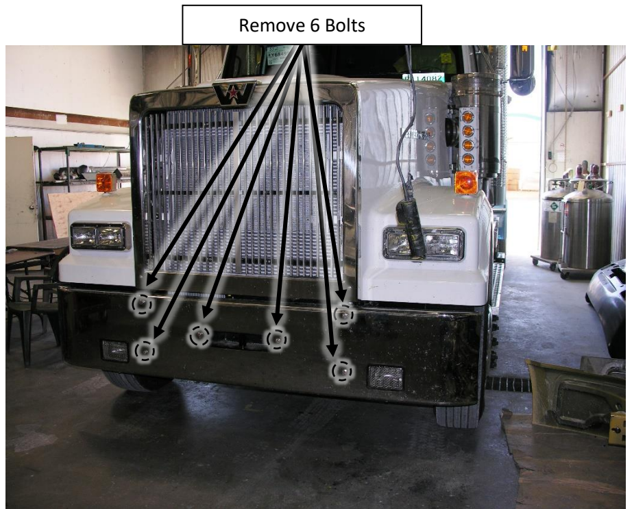
Figure 3 – OEM Bumper Removal Front View
